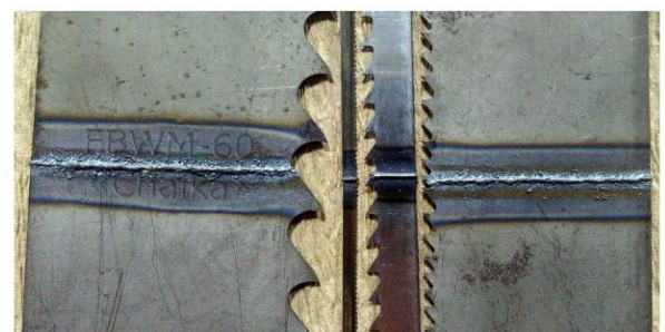
Flash Butt Welding
